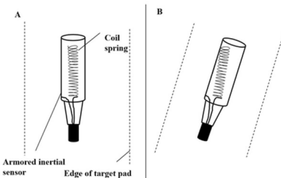
**Figure 2.** Coupled inertial sensor inside the target pad: (A) – before the kick contact; (B) – after the kick contact (closed electronic circuit between the coil spring and the armored inertial sensor).
