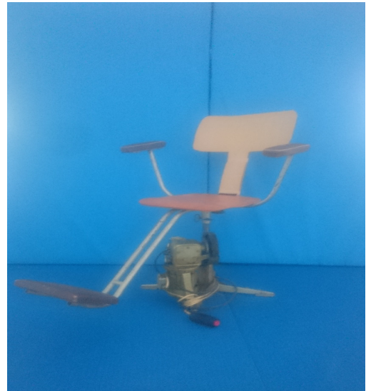
Figure 3. The Barany's swivel chair with an electric motor that serves to put the chair in a rotary motion.
