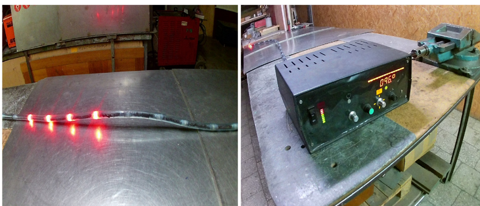
Fig. 1. The device "Lider" (Kuca Ltd., PL), consisting of a controller and polyvinyl chloride tube, (which includes LEDs) before installation at the bottom of the pool
