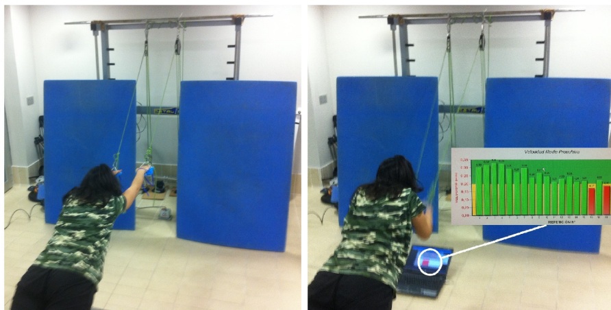
Fig. 1. The Smith Machine device showing both conditions (left: verbal feedback, right: visual feedback)
