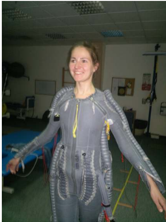
Fig. 1. WUK high altitude protection suit used in experiments (photo presented with patient's consent).
