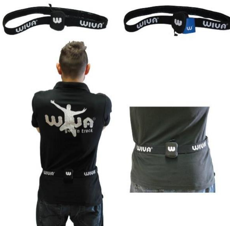
Figure 2. Correct positioning of the WIVA® System on the subject's spine.
