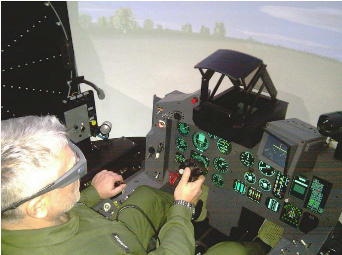
Fig. 2. A pilot (TG) during the oculography test in the human centrifuge.
