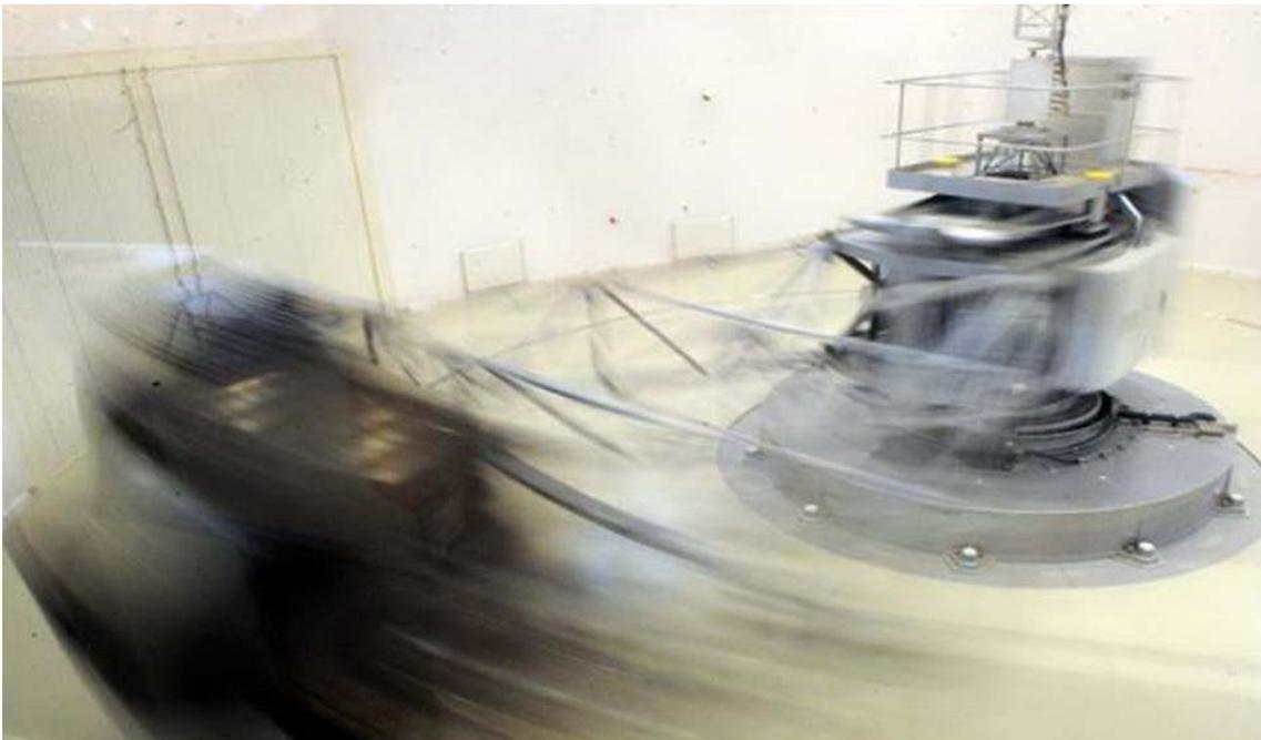
Fig. 1. Human centrifuge in motion.
