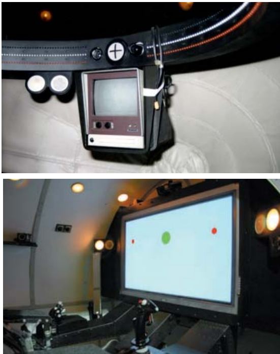
Fig. 9. Visual field meter (first on the left) installed in the centrifuge chamber.
