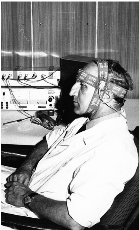
Fig. 8. Set up of the Doppler sensor to measure the blood flow rate at the temporal artery level.
