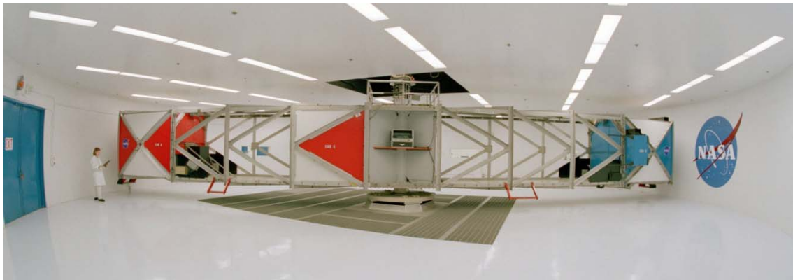
NASA Ames Human Centrifuge Configured with Cab A (left) and Cab B (right).
