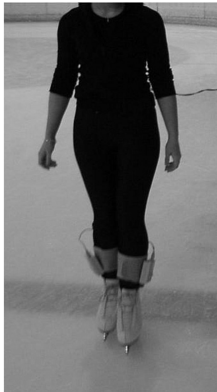
Fig. 1. A participant wearing the F-scan in shoe pressure system with cuffs attached about the lower shanks
