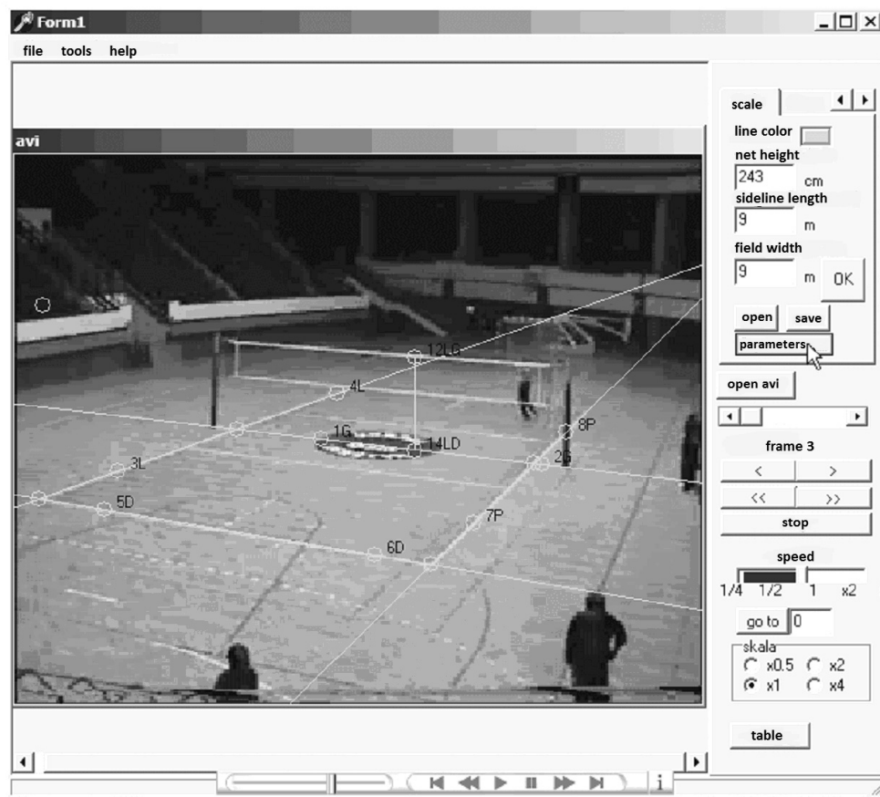
Fig. 3. The monitoring plane with marked points for identification of flat transformation in the AS-4 program
