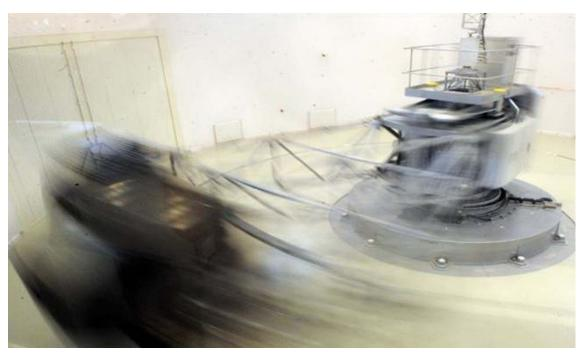
Fig. 1. Human centrifuge in motion.
