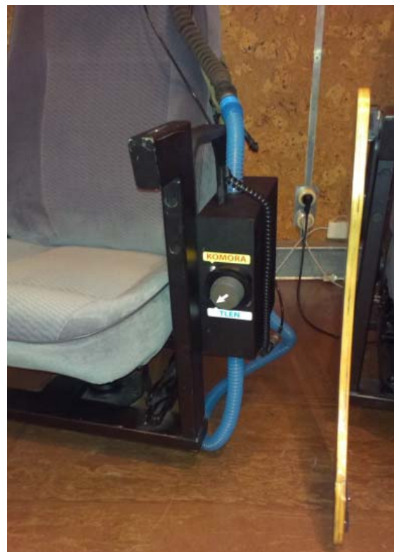
Fig. 5. Installation of the pilot's panel. (symbols: KOMORA = CHAMBER, TLEN = OXYGEN)
