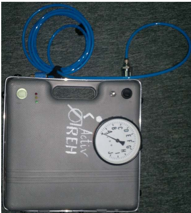
Fig. 8. The compressor for filling the R-WUK suit.
