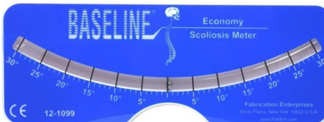
Figure 2. Bunnel's Scoliometer [own source].
