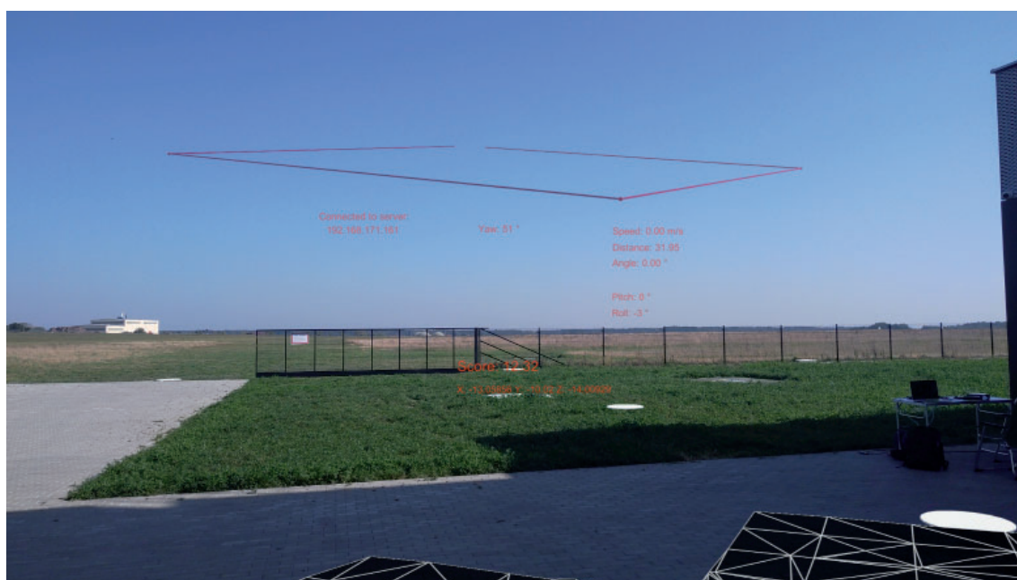
Fig. 16. Visualization of an exercise in the HoloLens 2 app, with the furthest corner of the guideline disappearing due to distance.
