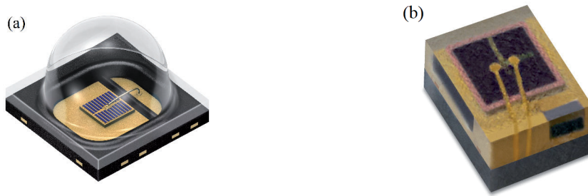
Fig. 3. SMT LEDs: (a) OSLO Black - OSRAM [1], (b) LUXEON IR Compact Line - Lumileds [16,17].
