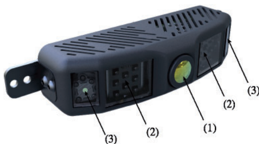
Fig. 2. OEM DMS module, (1) camera lens, (2) LED illuminator, (3) NIR VCSEL – GENTEX CORPORATION [11].
