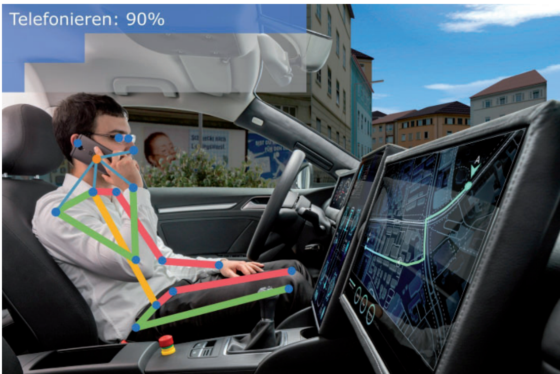
Fig. 1. Driver activity detection using skeletal key point analysis – Fraunhofer IOSB [40]
