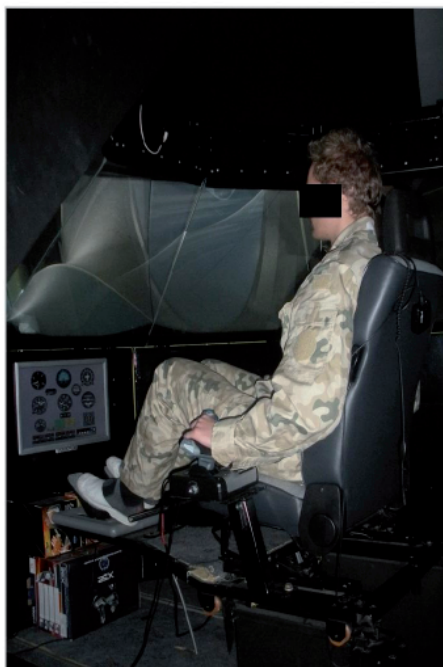
Fig. 2. A participant in a fixed-base flight simulator (A) equipped with a mirror-based collimated visual system (B), and display with primary flight instruments (C).
