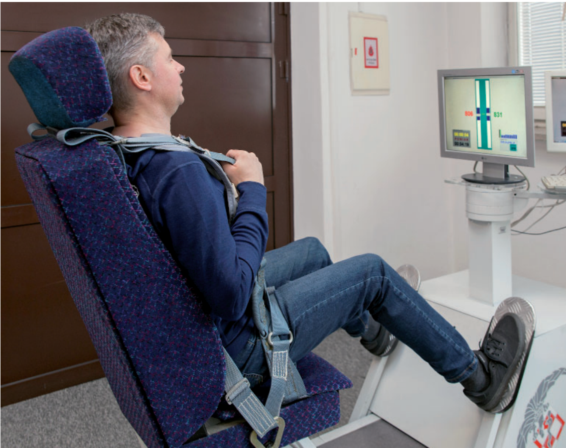
Fig. 1 Method of measuring lower limbs pressure force on the rudder pedals of the diagnostic-training stand (Source: Military Institute of Aviation Medicine).
